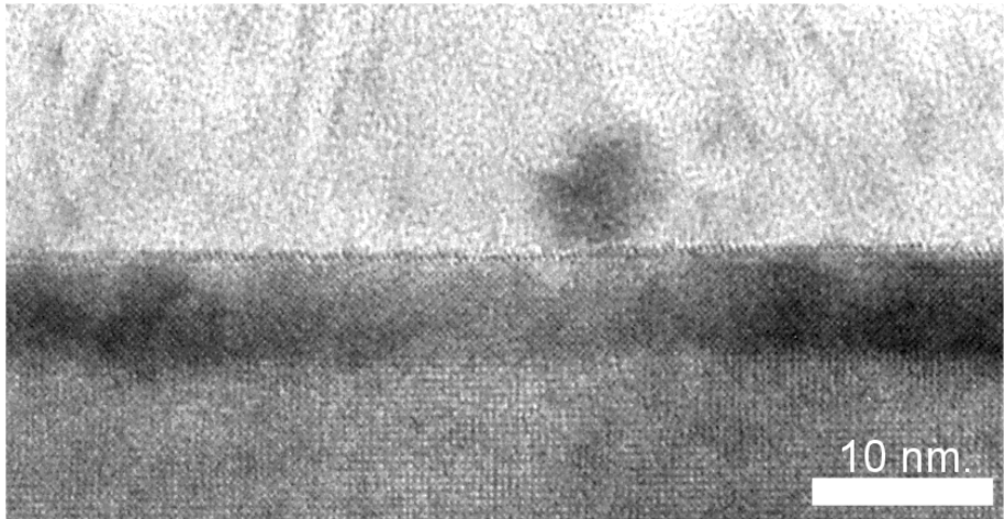
Figure 5.10: Cross-sectional TEM image of the same La 0.67 Sr 0.33 MnO 3 / SrTiO 3 / Co stack. With these TEM settings, the SrTiO 3 / Co interface does not show a white line.
